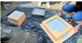
Fig. 9 Photos from the moment of making the scale foundation model.
