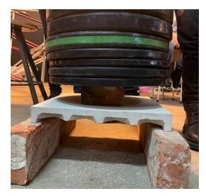
Fig. 4 Loading of the slab model
