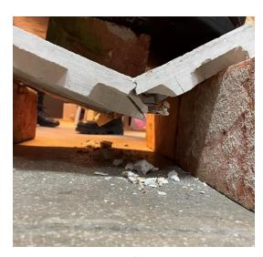
Fig. 5 Failure of the slab model
